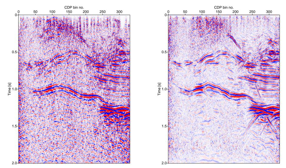
NMO/DMO/stack vs. CRS stack – 3-D data, inline A From Bergler et. al (2002). Data courtesy of ENI E & P Division.
