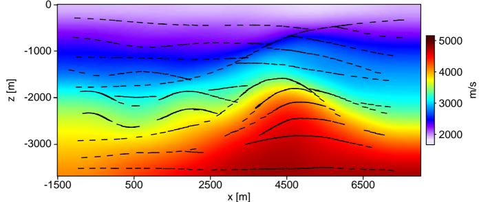
Original velocity and reconstructed reflector elements
