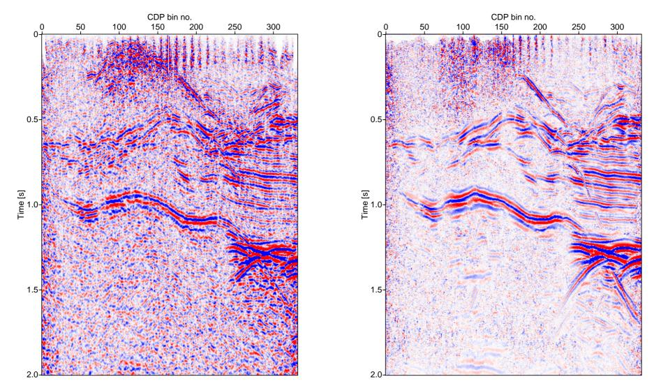
NMO/DMO/stack vs. CRS stack – 3-D data, inline B From Bergler et. al (2002). Data courtesy of ENI E & P Division.
