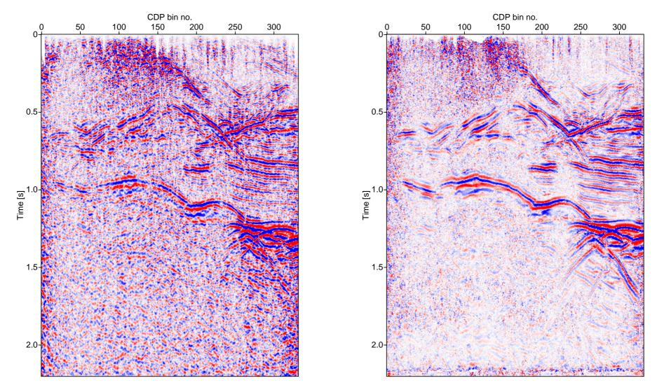
NMO/DMO/stack vs. CRS stack – 3-D data, inline C From Bergler et. al (2002). Data courtesy of ENI E & P Division.
