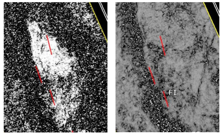
depth slices of coherence images: conventional vs. CRS-based Courtesy of ENI E & P Division
