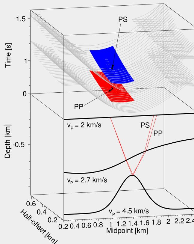
Figure 1: Lower part: a simple 2D model with homogeneous layers. Upper part: forward-calculated traveltimes of PP- and PS-waves reflected at the second interface (gray CO traveltimes curves). The CO CRS stacking surfaces for PP- and PS-waves associated with the two depicted central rays are visualized in red and blue, respectively. The near-surface velocity  $v_G$  at the receivers in Equation (1) has to be chosen according to the respective wave type.
