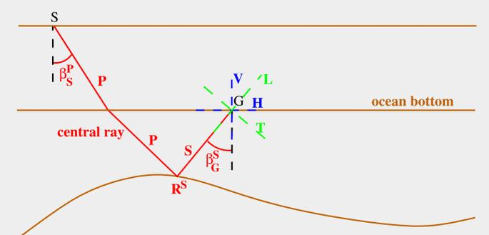
Figure 3: After the rotation of the vertical (V) and horizontal (H) components we obtain the longitudinal (L) and transversal (T) components. For the depicted case of a central PS-ray,  $\gamma$  coincides with  $\beta_G$ . Note that this strategy is not restricted to the OBS geometry illustrated here.
