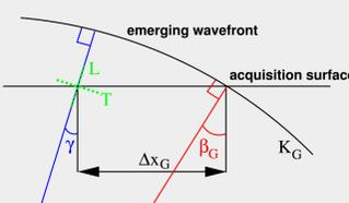
Figure 2: Definition of emergence angles for central (red) and paraxial (blue) ray. The expected transversal (T) and longitudinal (L) polarization directions are indicated in green. See main text for  $K_G$  and  $\Delta x_G$ .
