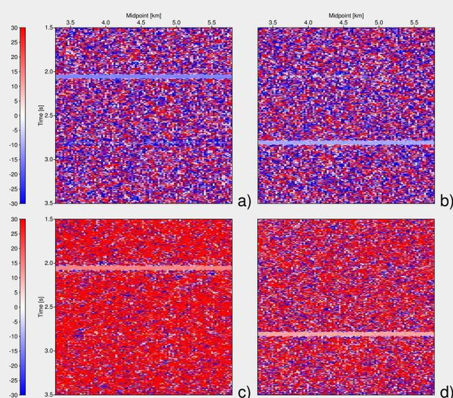
Figure 6: Kinematic wavefield attributes determined by the CO CRS stack. Upper part:  $\beta_G$ -sections [°] for a) PP- and b) PS-reflections. Lower part:  $\beta_S$ -sections [°] for c) PP- and d) PS-reflections.
