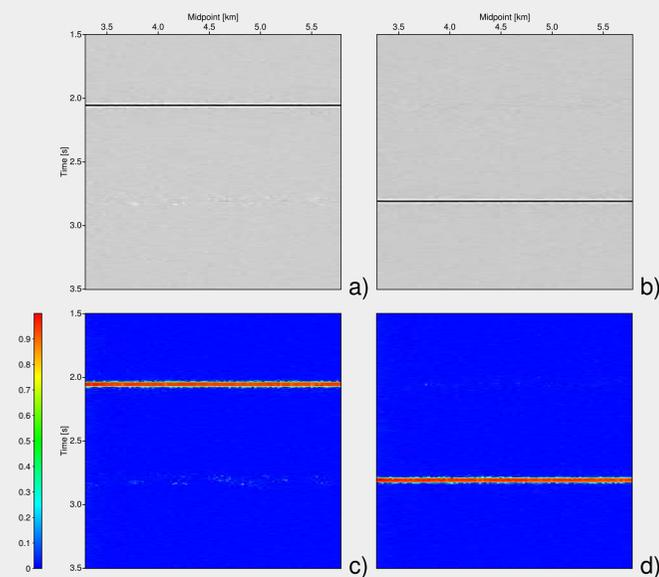
Figure 5: Upper part: a) PP and b) PS CO CRS stack section. Lower part: associated coherence sections for c) PP- and d) PS-reflections.
