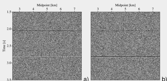
Figure 4: CO sections for half-offset  $h = -0.5$  km extracted from the synthetic prestack data: a) vertical and b) horizontal component. Both events can be observed on both components, the upper event is the PP-reflection, the lower the PS-reflection.
