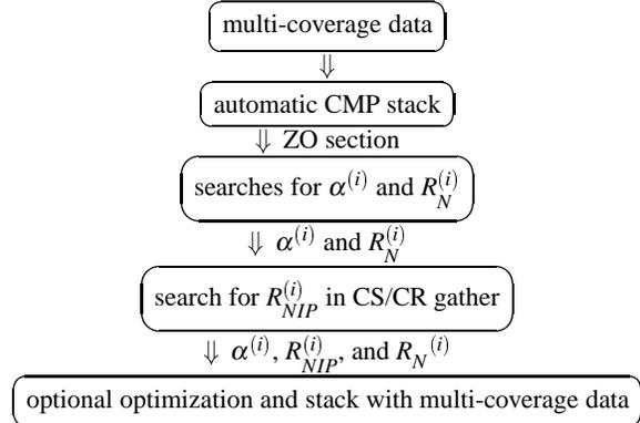
Fig. 3: Simplified flowchart of the adapted search strategy. The index  $i$  denotes the different events detected for one and the same ZO sample.
