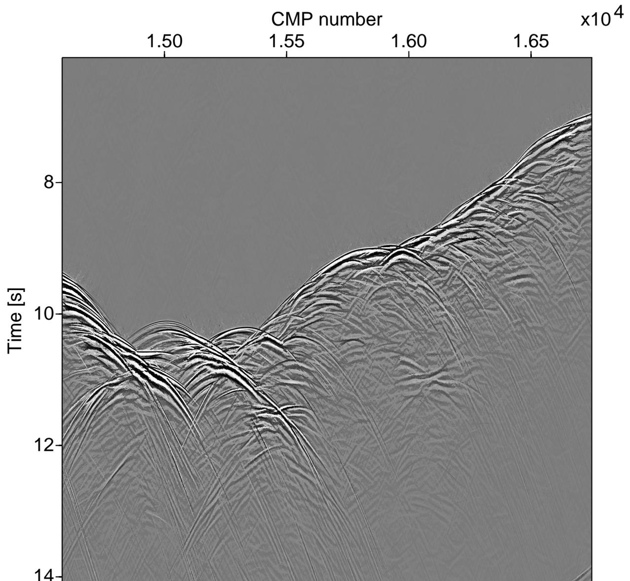
Figure 1: Zero-offset section simulated with the common-reflection-surface stack method.
