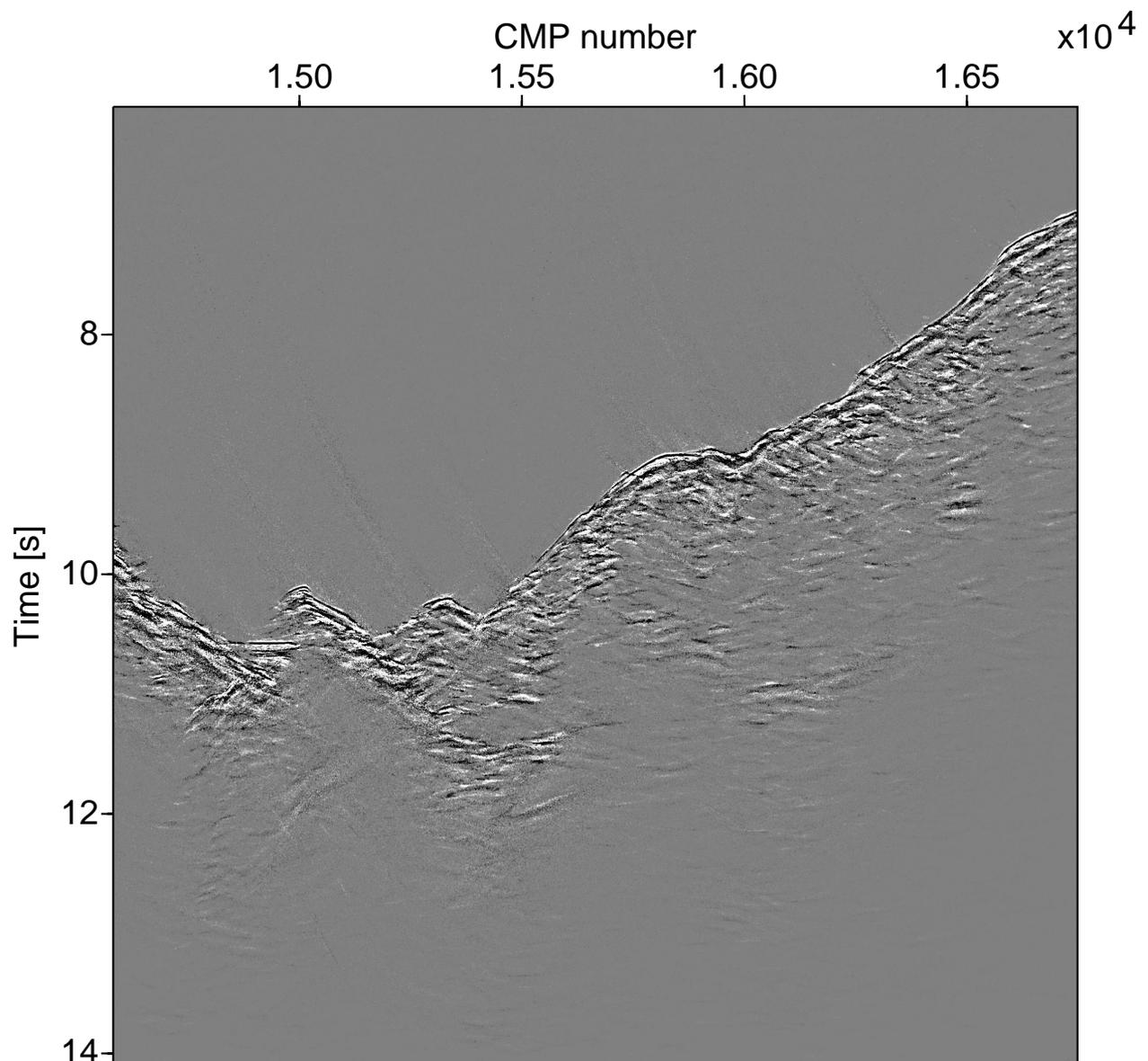
Figure 2: Result of the approximative pre-stack time migration based on CRS wavefield attributes.
