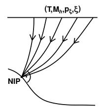
In consistent velocity models, NIP waves focus at zero traveltime.
