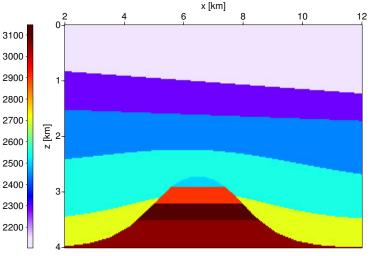
interval velocity [m/s] model at y = 5000 m
